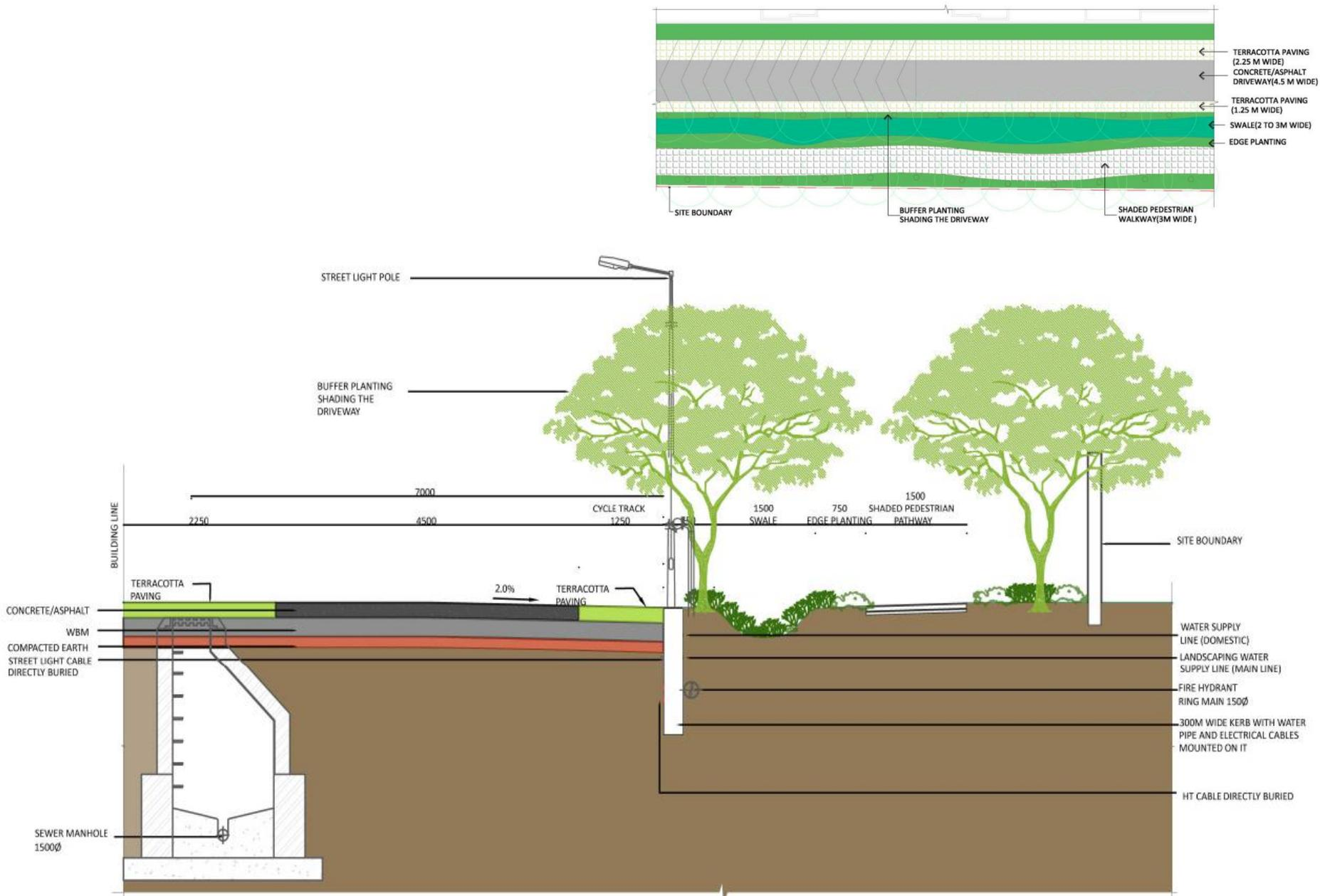
Section 01: High Traffic Loop Roads (Concrete Roads) with swale
