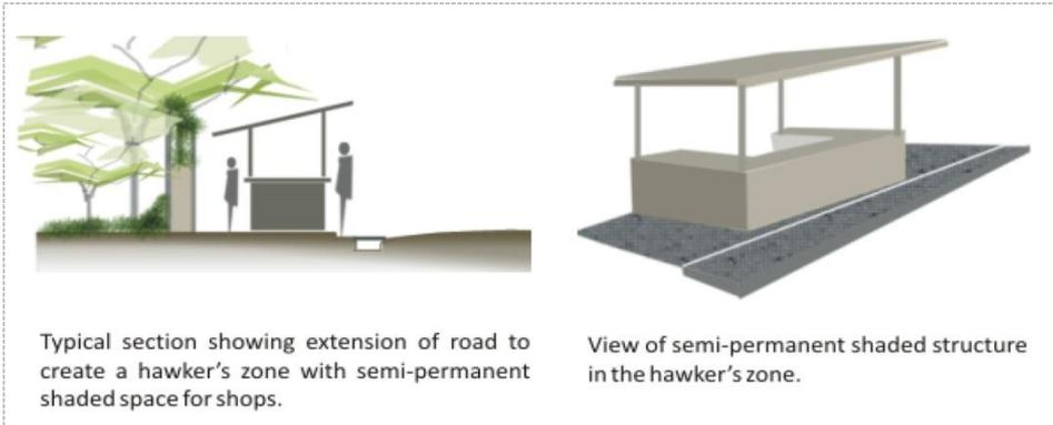
Typical section showing extension of road to create a hawker's zone with semi-permanent shaded space for shops.
