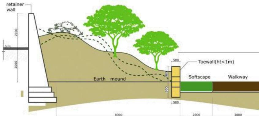
SECTION 01 : Section of earth berm along highway edge
