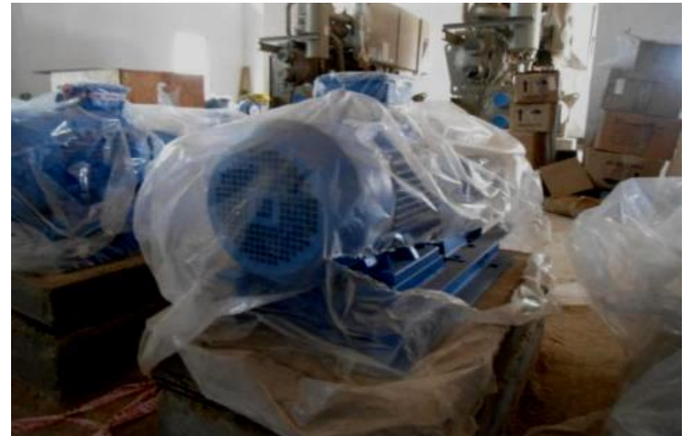
Protection of MEP Equipments, Materials etc. Being procured at site
