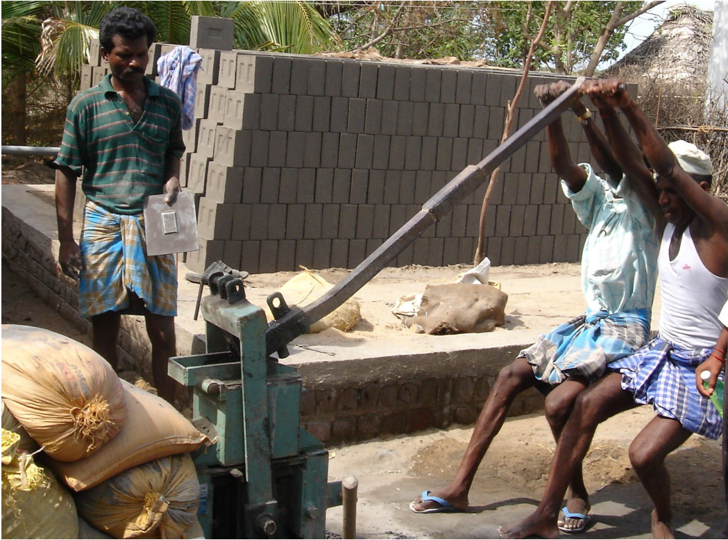
Block Production (manual process)
