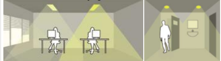
Combination of Daylight & motion detector
