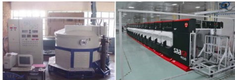
Large Area MgO coating Unit for Santel 1 m x 1 m PECVD for a-Si solar modules
