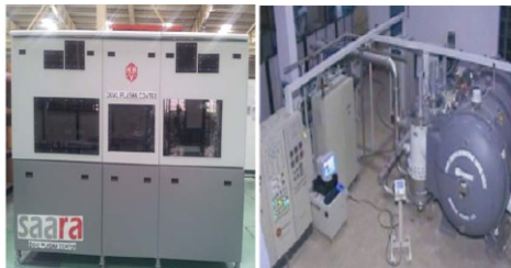
Dual Plasma Coater for Solar Thermal coatings Multi-Axis Robotic Coater for Canopy
