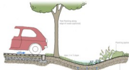
Open Standard Swale. Percolation 10%, Other Losses= 30%
