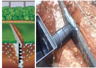
Strip Drains to increase surface water and sub surface water collection
