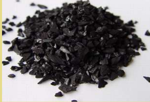
Activated carbon granules
