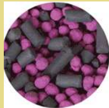
Activated carbon pellets and \text{KMnO}_4 impregnated on alumina mixed together
