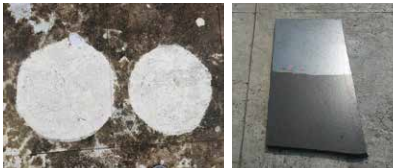
» Figure 4: Pictures of nano \text{TiO}_2 coated on terrace and tile exposed to three rainy seasons
