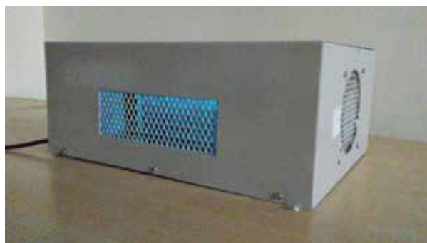
» Figure 3: Photocatalytic air purifier developed by EnviPure using TiO 2 nanostrands coating specifications
