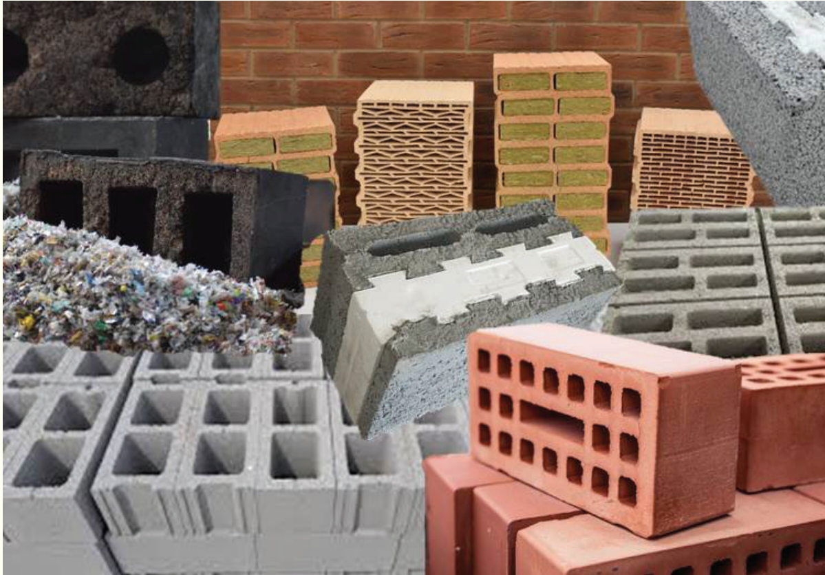
Image 2: Some examples of new-age bricks available in the market: ceramic bricks, recycled plastic bricks, hollow AAC blocks and self-insulated composite blocks
