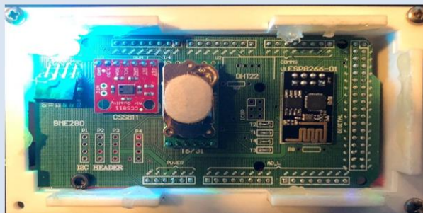
At the centre of each myair is a precision Telaire T6713 CO 2 sensor.
