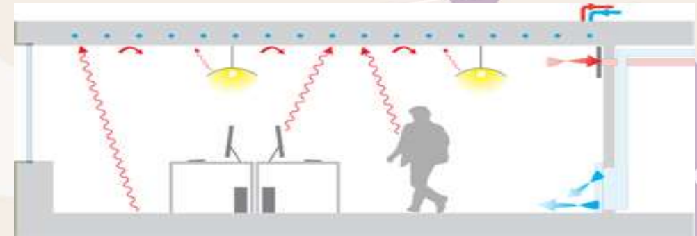
Fig: A room cooled with a high mass radiant ceiling slab. The slab is absorbing heat radiated from the people, surfaces, equipment, and lights in the room.
