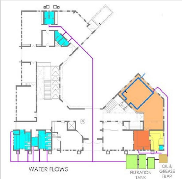
FLOOR PLAN SHOWING THE BASIC PLUMBING LINES
