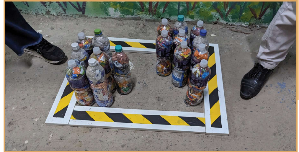
▲ Plastic bottles being used to create masonry units
