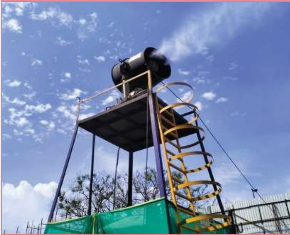
▲ Spray gun being used to spray water on to the fine material
