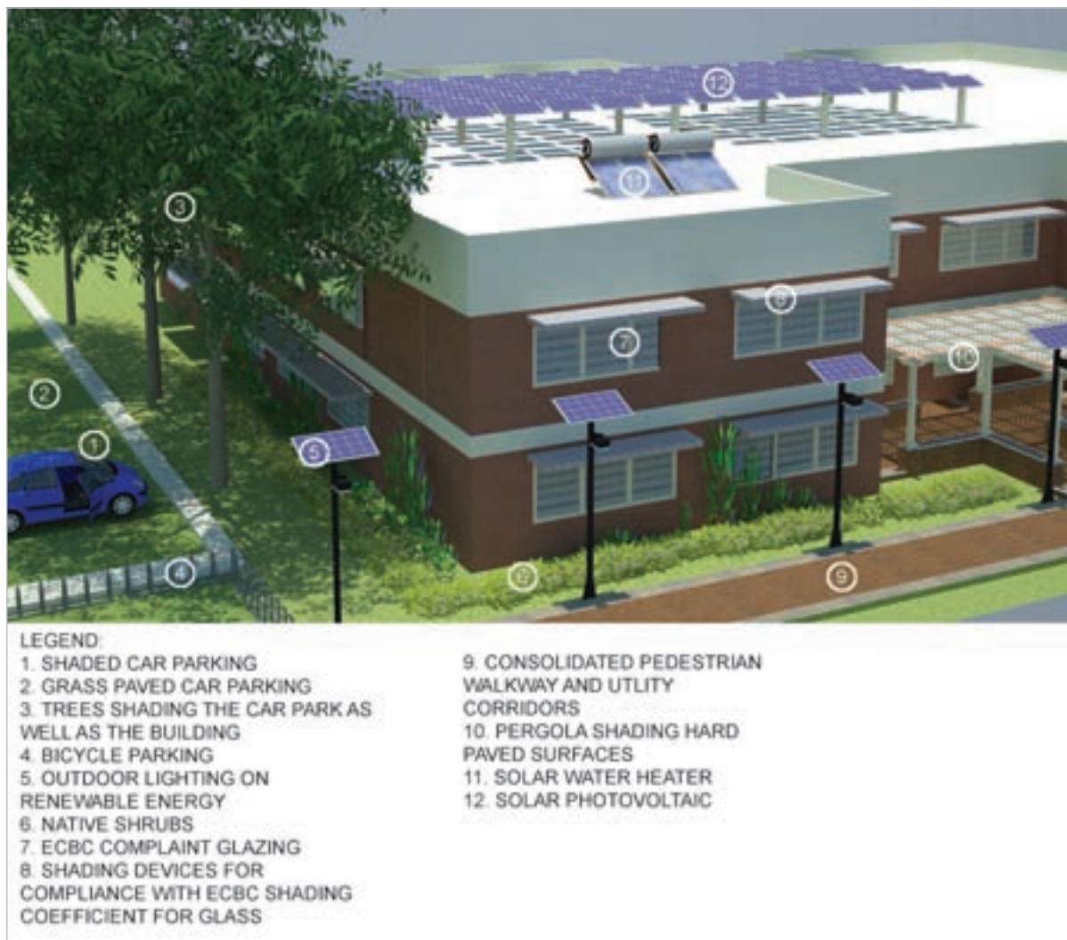
Figure 1 Schematic diagram highlighting select green building features
