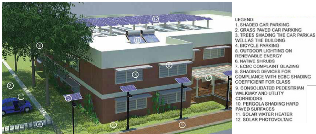
FIGURE 5: Schematic diagram highlighting green building features
