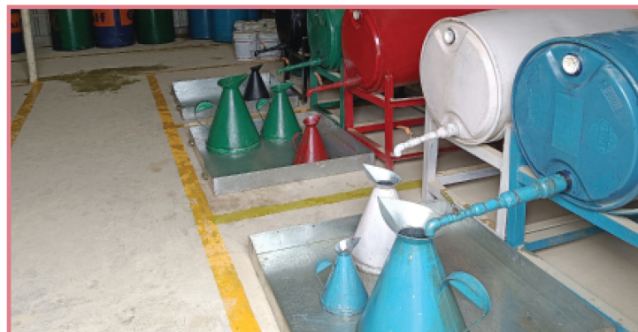
▲ Hazardous material stored on impervious land
