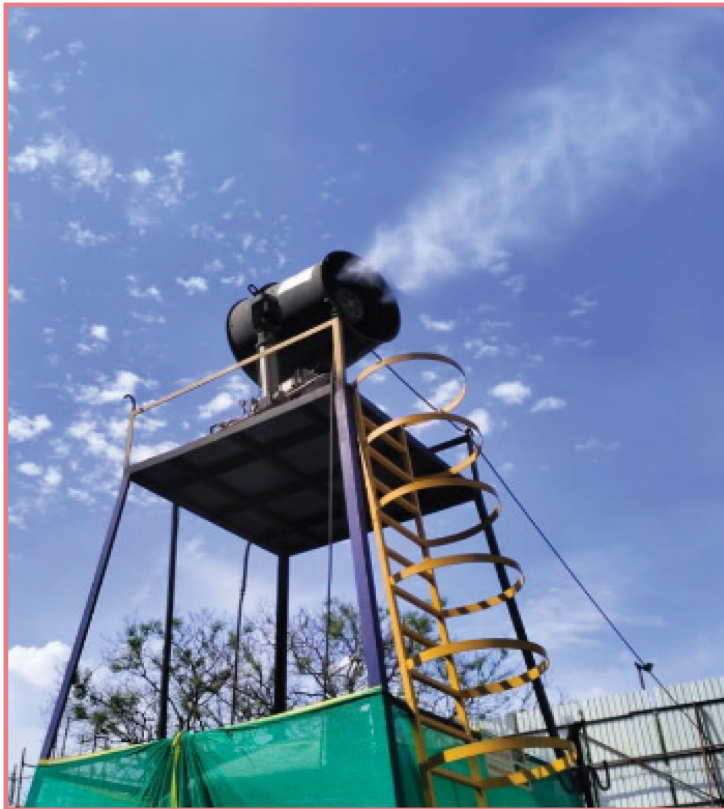
▲ Spray gun being used to spray water on to the fine material
