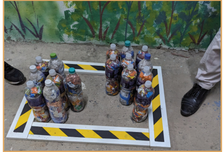
▲ Plastic bottles being used to create masonry units
